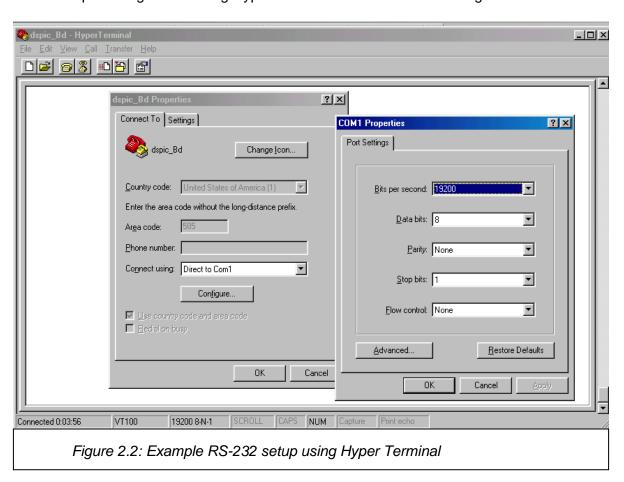
In the default state, the RS-232 port will echo the same information sent to the front panel LCD display, allowing a running datalog to be stored to disk using the capture feature of the terminal program.
